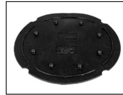
Pedestal Buffer Pad: Provides protection to waterproofing membrane from wear and provides slip resistance to pedestal. Attaches to bottom of base. Align perimeter notches with chalk lines.
