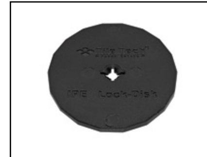
IPÊ Lock Disk: Used to secure wood tiles by inserting disk into kerf-cut between the upper slat and bottom rail, adding the 4th tile and securing with 1-1/4" deck screw.
