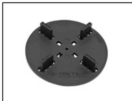
Spacer 1/8" (3mm): Used with wood deck tiles or porcelain pavers without trays. Allows for 1/8" spacing gap between pavers for drainage. Tabs are perforated for easy removal.
