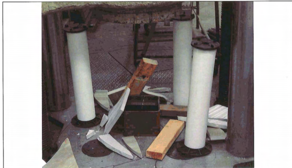
Photo No. 2: General view of Porcelain Samples Failure
