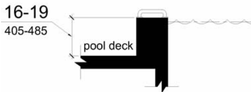
Fig. 75 Transfer Wall Height
